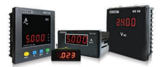
Digital panel meters available in 96x48 and 96x96 sizes. Single phase as well as 3-phase models with 4 digit ultra bright LED display. These meters are micro-controller based design with site programmable PT ratio and True RMS measurement. 3 1/2 digit modules.
