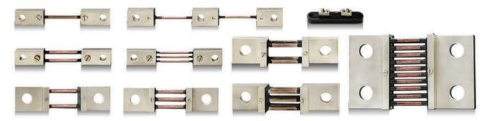
Available in a wide range from 1A - 25,000A, our Ammeter Shunts are manufactured with high quality Manganin wire, which is the best alloy for shunts application with temperature coefficient of only 10ppm. This provides a high level of stability. Our shunts are available in rod and fin configurations. Bakelite base is available for certain models.
